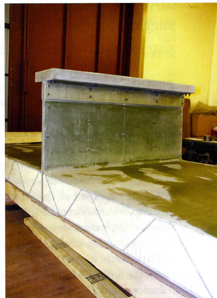
Fig. 1 – Part of LNG carrier's tank wall to wind the same simultaneously with cylindrical section. Even best variants with included compounds are less efficient, than single structure of cylinder and isotensoid.
