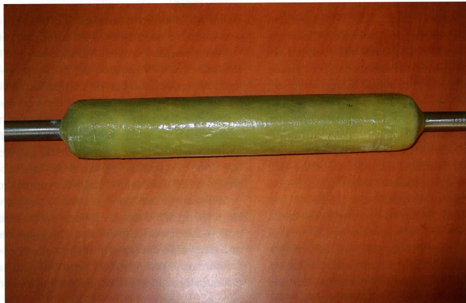
Fig. 4 – Insulation device with channels
